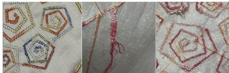
Fig. 10. Variety of stitch tension problems
